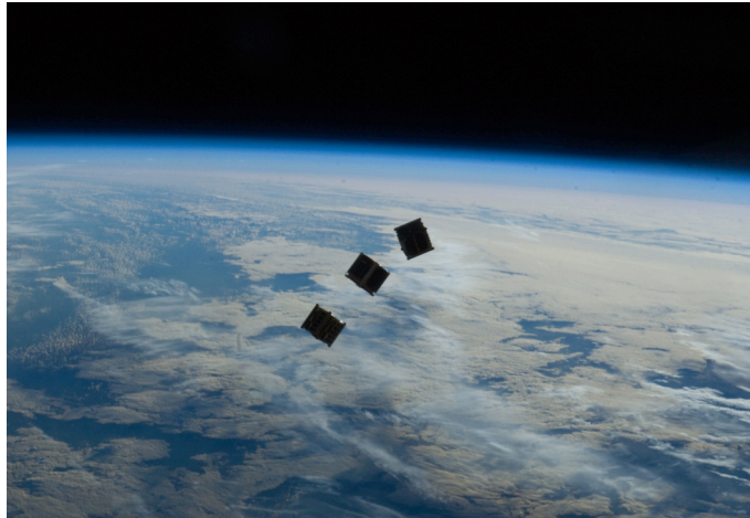
Figure 4: Three CubeSats in low-Earth orbit just after deployment from the International Space Station (Credit: NASA)
