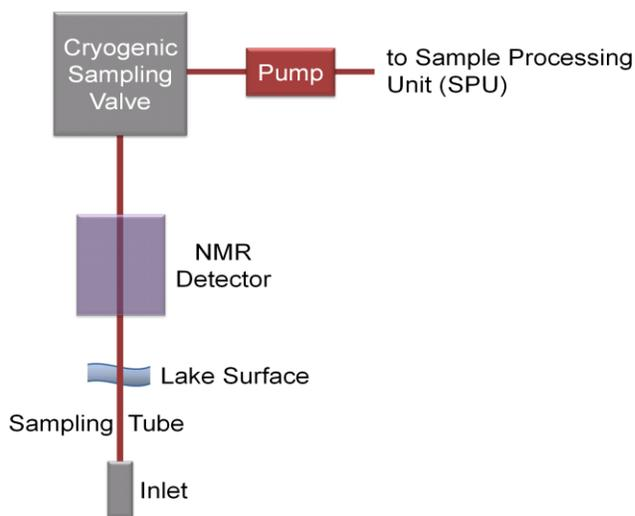
**Figure 4-3.** Example of a cryogenic liquid sampling system for Titan lakes.
