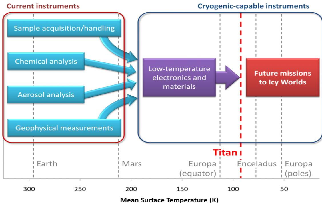
**Figure 4-14.** Goal of KISS study in terms of electronics and materials. All current instruments required for (1) sample acquisition and handling, (2) chemical analysis, (3) aerosol analysis and (4) geophysical measurements which have been designed to operate at Earth or Mars ambient temperatures, must be adapted to operate in the cryogenic conditions of the Titan environment (red dashed line). This will enable future missions to other icy worlds such as Europa and Enceladus.
