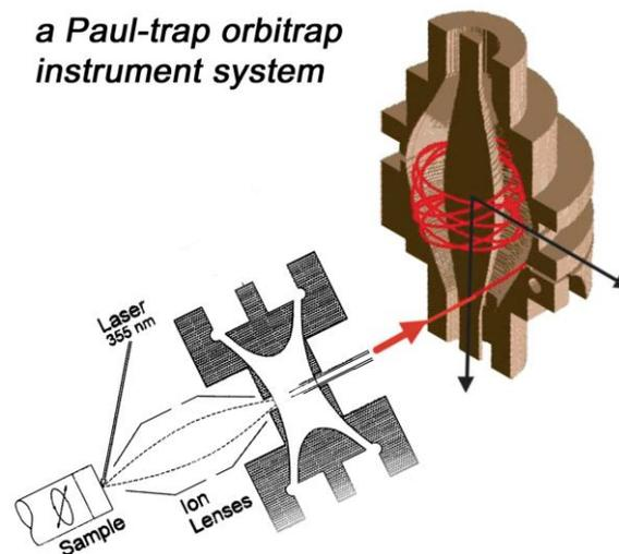
**Figure 4-8.** Concept for a Paul-trap Orbitrap system, where fast injection of ion packets into the Orbitrap is achieved using a Paul-trap instrument as a 'front end' to the Orbitrap mass analyzer. Image from Hu *et al.* 2005.<sup>29</sup>
