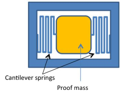
**Figure 4-11.** Schematic of a double cantilever MEMS seismometer design.<sup>74</sup>
