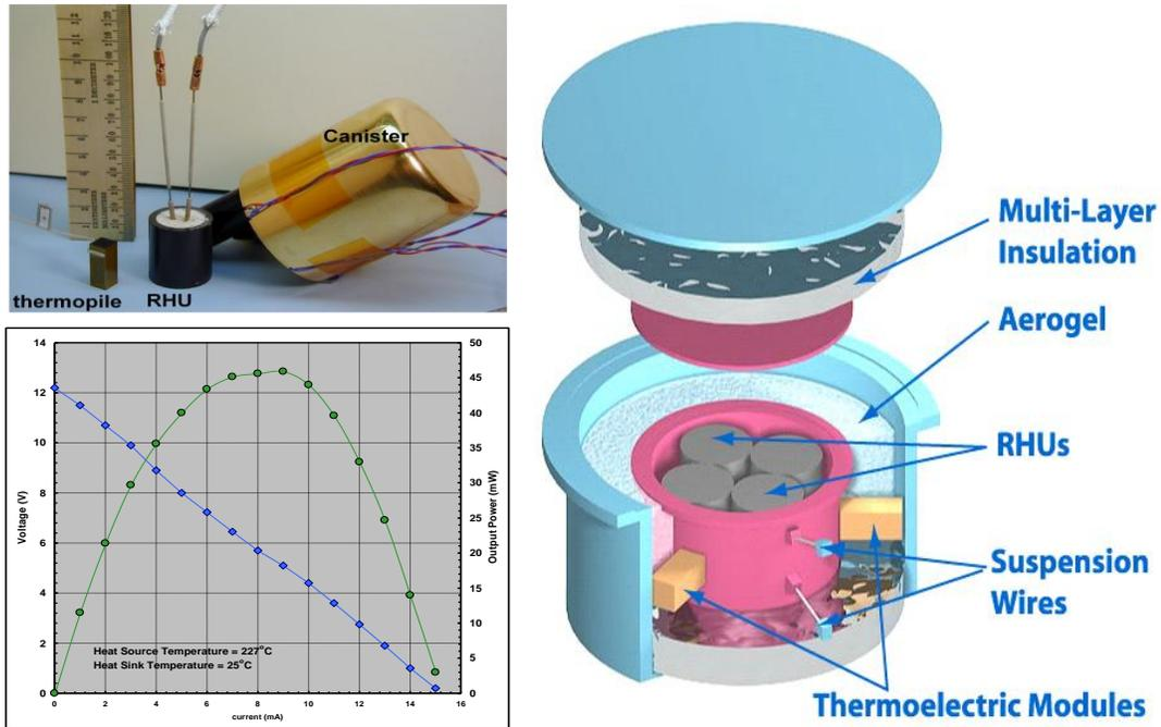
**Figure 4-16.** Micro RTG and its characteristics. Top left: Photo showing scale of micro RTG. Bottom left: Current-voltage-power characteristics of micro RTG; voltage (V) in blue, output power (mW) in green (heat source 227 °C, heat sink 25 °C). Right: Diagram of components of micro RTG.
