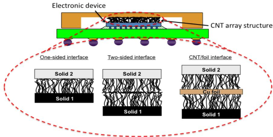
**Figure 4-19.** Potential packaging arrangement using CNT arrays
