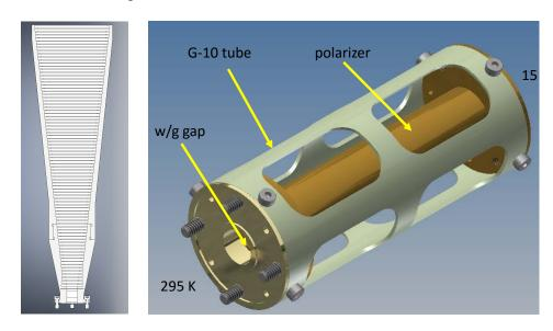
Figure 2: COMAP corrugated feedhorn (left) and circular polarizer (right)
