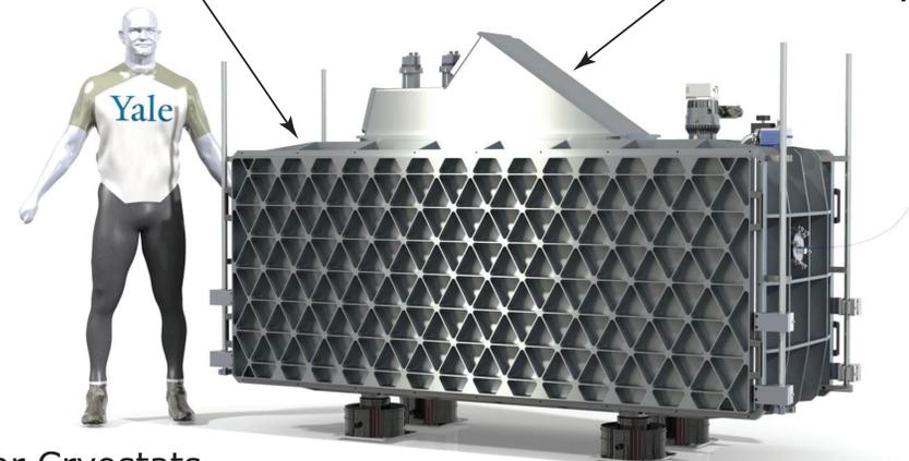
Detector Cryostats & Pulse Tube Coolers
