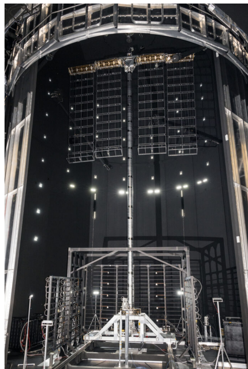
Figure 5.1: Thermal Vacuum Testing of LAMPS at NASA Johnson Space Center. (Photo credit: NASA/David DeHoyos)
