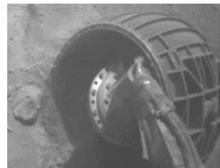
Figure 4-7: The MER Spirit's right-front wheel failed on sol 778.
