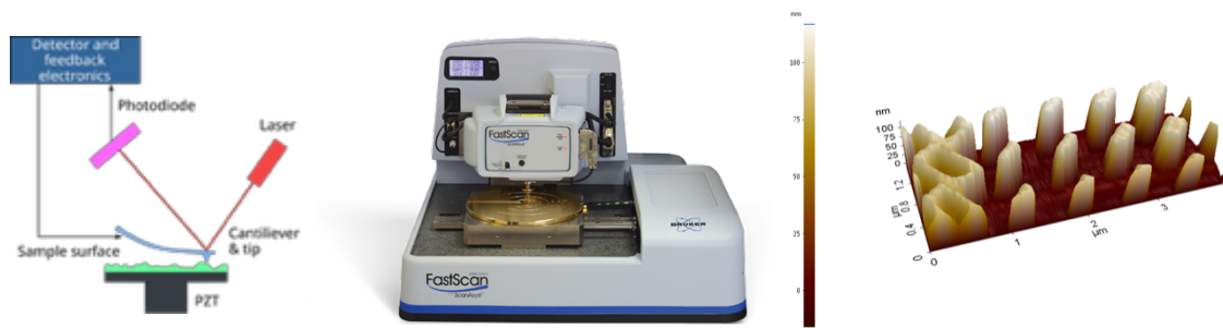
Figure 6.2. (Left) The fundamental operation of the AFM. (Center) A laboratory instrument. (Right) Sample data of a metasurface. Image credit: Bruker Corp.
