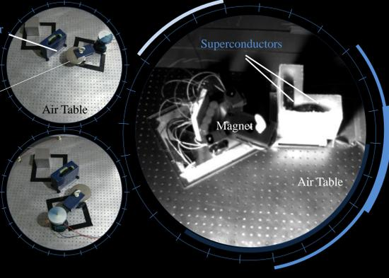
System-level laboratory testing enables FPI prototypes to improve their traceability-to-flight, by developing into higher-fidelity test articles such as the CubeSat-scale FluxCraft (below). FluxCraft integrate wireless communications, on-board sensing and actuating capabilities, and solid thermal and structural designs intended to mimic the flight requirements for an orbital CubeSat-scale FPI.
