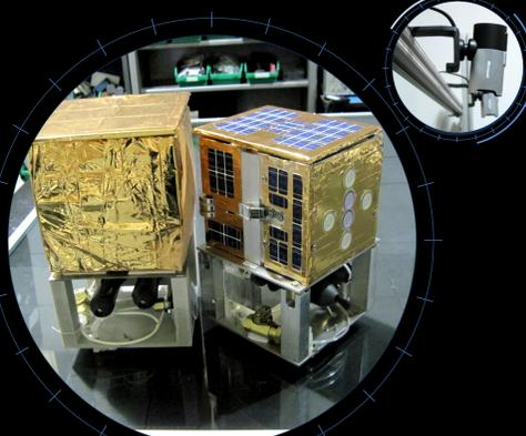
The FloatCube testbed consists of a structure with air feet bearings and CO<sub>2</sub> cartridges to provide a reduced-friction testing environment for the FluxCraft satellite mockups. An overhead camera system can collect real-time data from the platform.
