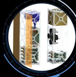
One proposed orbital FPI demonstration would use the CUSat nanosatellite bus with two non-contacting segments whose relative dynamics are influenced by flux-pinning physics.
