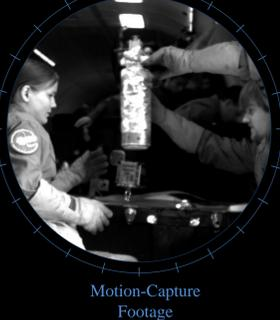
A 2009 NASA flight successfully demonstrated a flux-pinned revolute joint for the first time in microgravity using a prototype satellite mockup and a free-floating dewar of liquid nitrogen containing superconductors.
