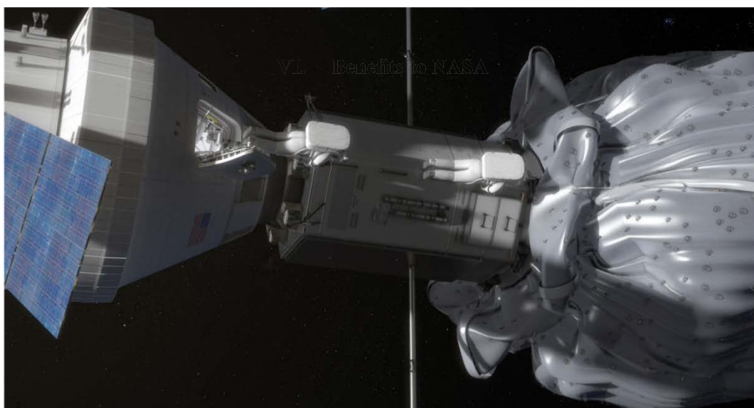
Figure 8. Illustration of the first crewed mission to the asteroid delivered to a Lunar Distant Retrograde Orbit (DRO). The asteroid is in the capture bag to the right of the picture and the astronauts are shown traversing the body of the ARV.
