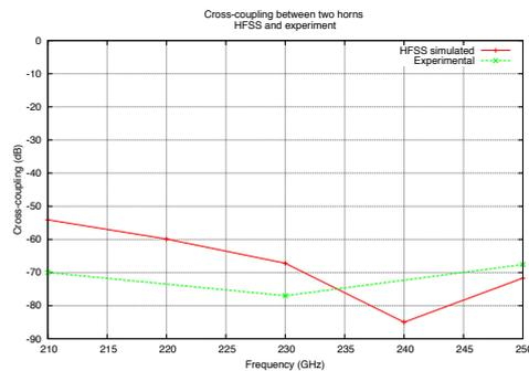
Figure 5: Measured and HFSS simulated cross coupling between the two horns in the 2 horn prototype array.
