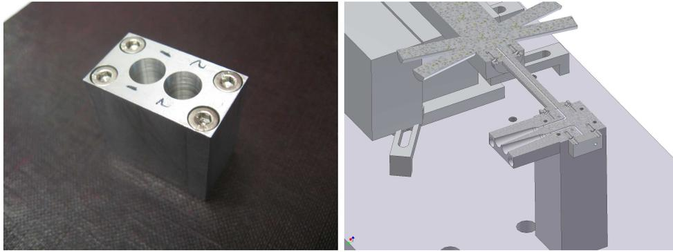
Figure 2: Left – The two horn array prototype, made by repeated drilling into a single block of aluminium. Right – a solid CAD model showing the two horn array and interface waveguide block.
