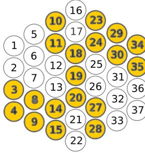
Figure 9: Schematic of the horn array highlighting the sample of horns tested.
