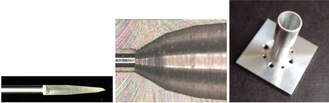
Figure 1: Left – the machine tool used for the fabrication of the drilled horn prototype, centre – the horn throat region and right – the finished single horn.
