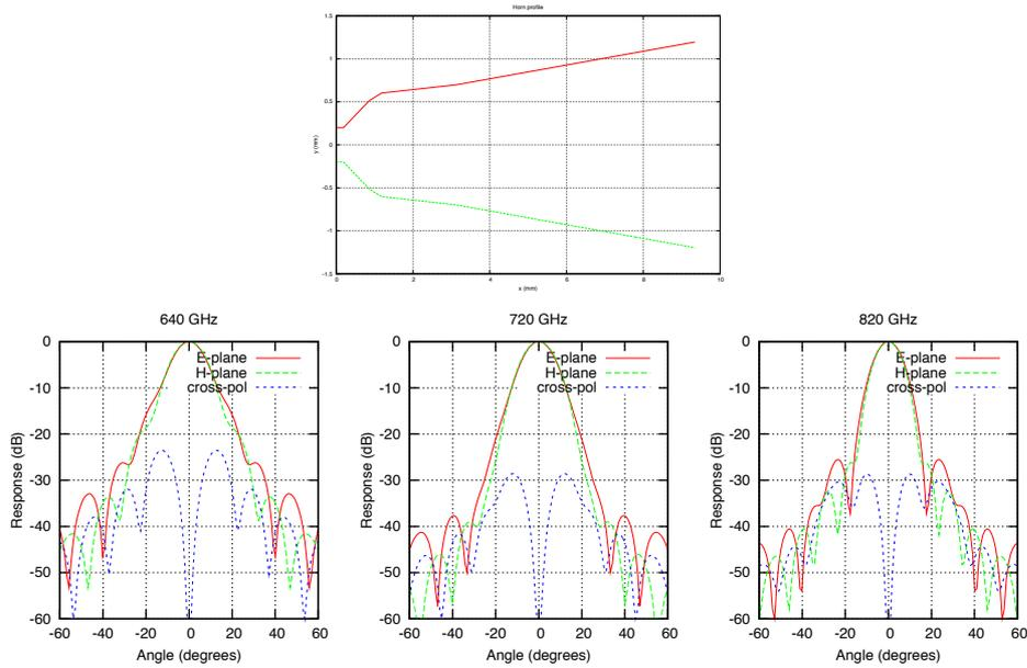
Figure 14: Top: Profile of a new horn design designed with our GA software for extended bandwidth. Bottom: Simulated beam patterns for this horn design. The fractional bandwidth illustrated is 25%.
