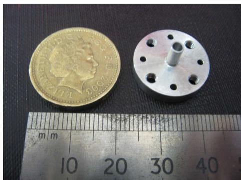
Figure 12: The 700 GHz drilled horn prototype.
