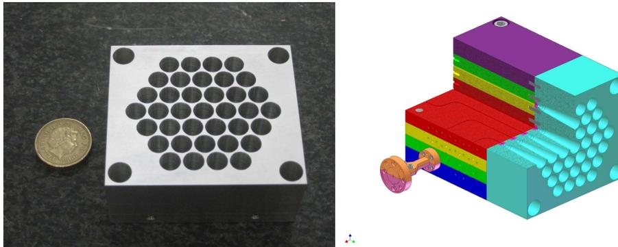
Figure 8: Left – The 37 horn array prototype, made by repeated drilling into a single block of aluminium. Right – the multiplate split block which enables power to be delivered to each of the horns from a split block waveguide at the side.
