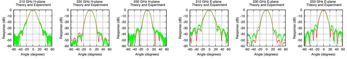
Figure 6: A comparison of the theoretical beam patterns calculated using modal matching and the experimentally measured beam patterns for horn No.1 of the 2 horn block (Left: H-plane, Right E-plane).
