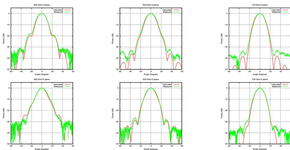
Figure 13: Experimental and theoretical beam patterns for the 700 GHz prototype horn Top: H-plane, Bottom: E-plane.
