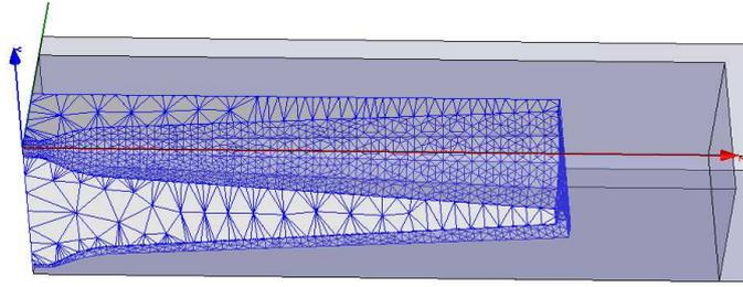
Figure 3: A section of the HFSS model used to calculate the cross coupling between two horns, showing the mesh points used.
