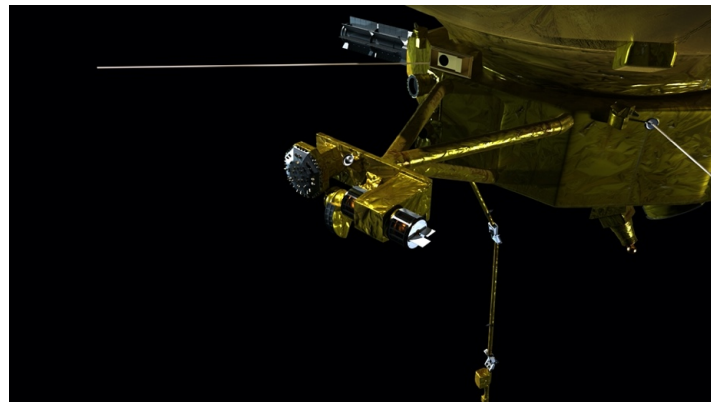
Figure A-17. VIR and IRM shown above the particle suite boom, respectively. They are pointed 90^\circ to the spacecraft ram direction. (Image credit: Johns Hopkins Applied Physics Laboratory.)
