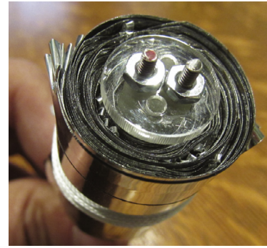
Fig. 26. Model #2 wrapped around the plug. The packaged diameter was 23.9 mm.
