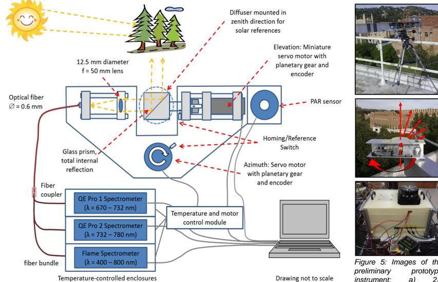
Figure 4: Top-view sketch of the instrument with the option to change azimuth and elevation viewing angles using a 2D scanner driven by servo motors.
