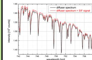
Figure 6: Example for a reference diffuser spectrum (black) and a diffuser spectrum plus an artificial SIF signal (red).
