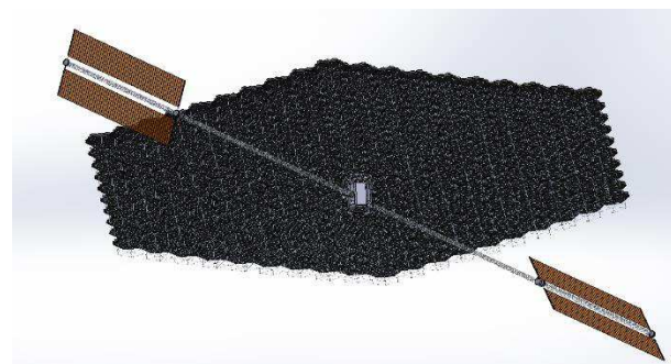
Fig. 2: Fully assembled primary mirror with central spacecraft and solar panels.
