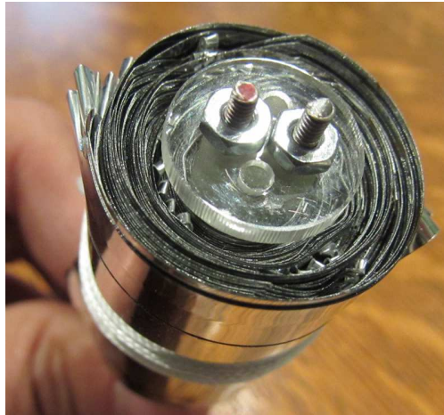
Figure 12: Model 2 wrapped around the plug. The packaged diameter was 23.92 mm.
