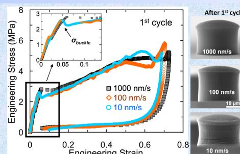
Tests at slower displacement rates show more pronounced buckling signatures and lesser recovery.
