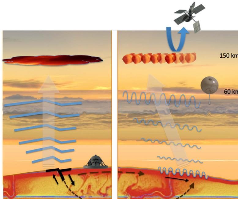
**Figure 4-10.** Propagation of seismic waves from source to point of observation. Waves propagate directly upward above the epicenter and also propagate as Rayleigh waves, which couple into infrasonic waves with increase in amplitude as they travel upwards in the atmosphere.
