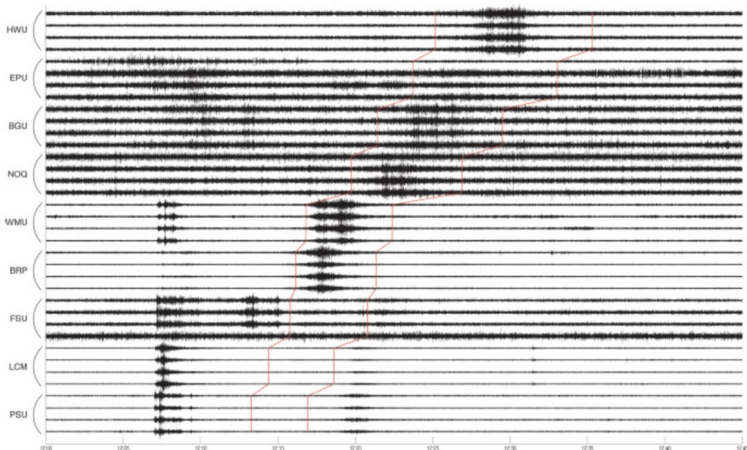
**Figure 6-2.** Centerville earthquake 2011. Signals from the nine stations in the University of Utah array are shown. This is filtered data in the 1 to 5 Hz passband.
