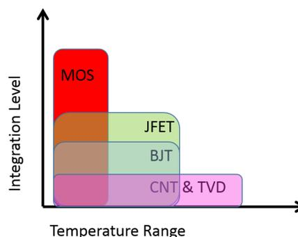
**Figure 5-6.** Integration for various kinds of active devices. The metal oxide semiconductor (MOS) and junction field effected transistor (JFET) are both silicon devices. The bipolar junction transistor (BJT) can be made with high band gap silicon carbide and the carbon nanotube (CNT) and thermionic Vacuum tube (TVD) are both vacuum electronics devices.
