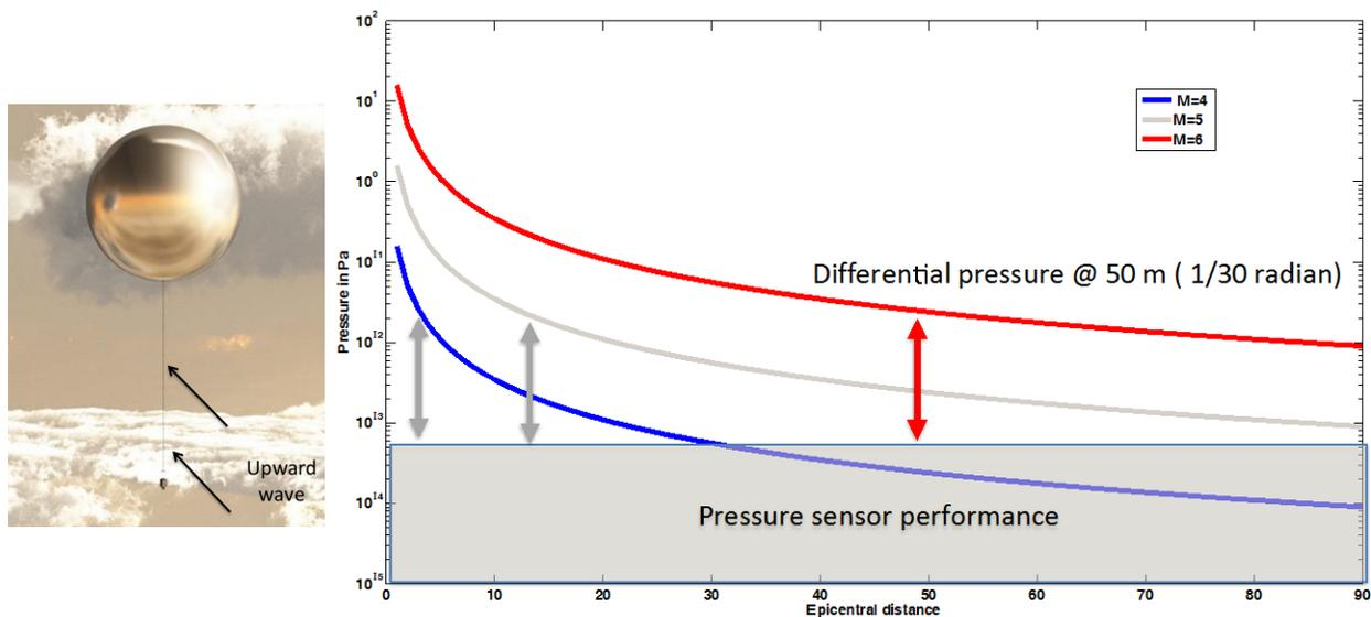
**Figure 6-9.** Right: Use of two barometers enables spatial filtering. Left: Differential pressure for a 50 m separation of the two barometers, as a function of the epicentral distance and for various earthquake magnitudes, at an altitude of 60 km. Atmospheric attenuation not taken into account. The shaded gray areas is the blind zone of an off-the-shelf differential barometer.
