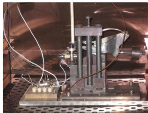
**Figure 5-5.** A prototype of a high temperature seismometer.
