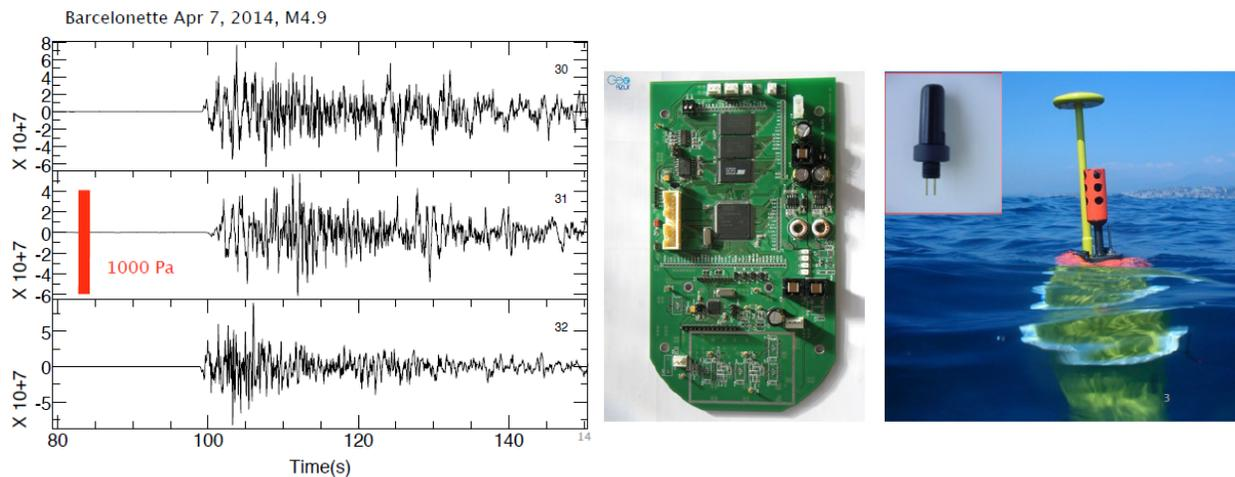
**Figure 6-3.** Left: Recording of an M=4.9 quake at  $\approx 150$  km. Right: MERMAID buoy data logger and hydrophone.
