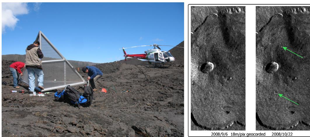
**Figure 7-8.** Orbital observations. *Left:* deployment of a radar reflector. *Right:* Reflectors seen from orbit.
