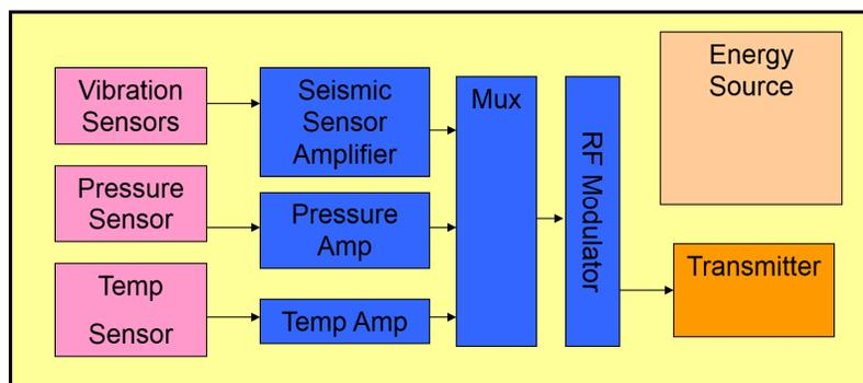
**Figure 5-9.** Block diagram of a completely analog seismometer for Venus surface operation. This does not require either an analog-to-digital converter or a digital memory, which are both challenging developments for high-temperature electronics technology.
