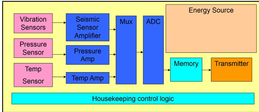
**Figure 5-8.** Block diagram for a concept of a digital seismometer with memory. All components must operate at Venus-surface ambient.
