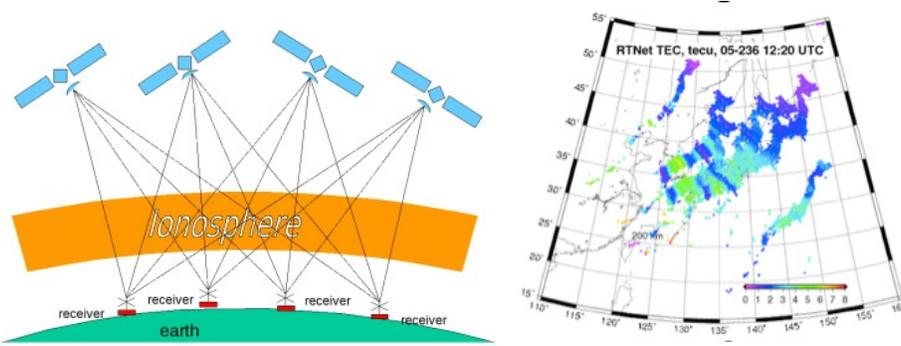
**Figure 7-2.** Ionosphere tomography measurement principle and resulting TEC map over Japan ([http://gpsmet.com/gps\\_ionosphere\\_space\\_weather.php](http://gpsmet.com/gps_ionosphere_space_weather.php)).
