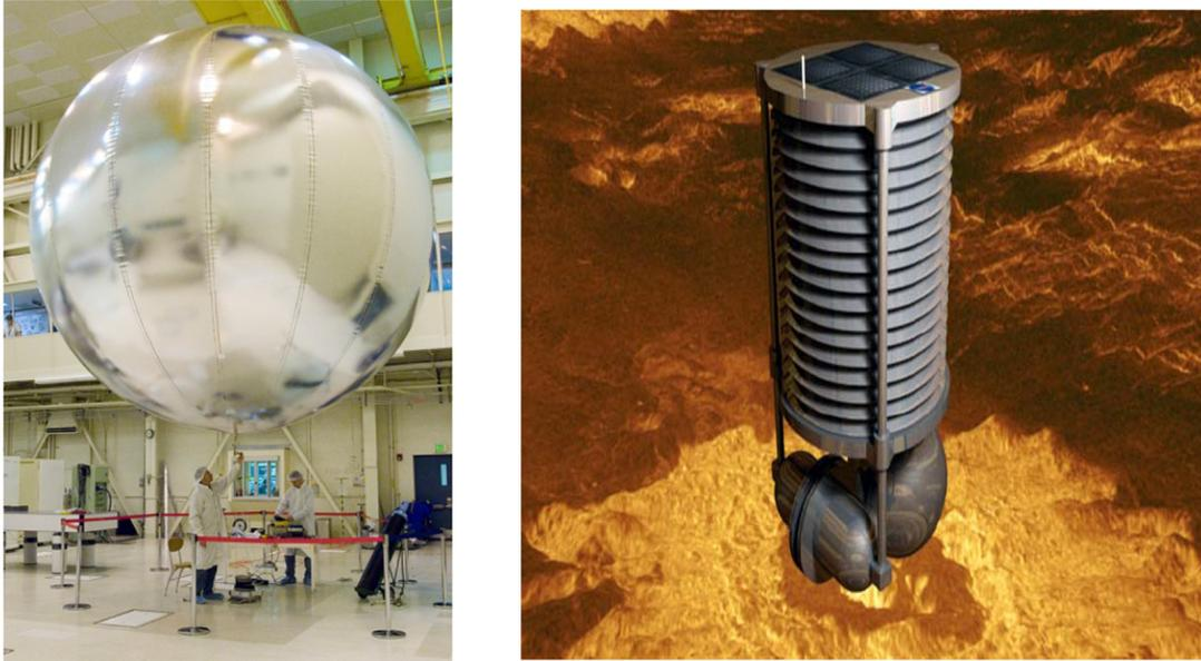
**Figure 6-8.** Flotation devices for the mid-cloud level on Venus (left) and for near surface operations (right). The two concepts have similar payload capacity but the vehicle on the right has only 2% of the volume of the balloon.
