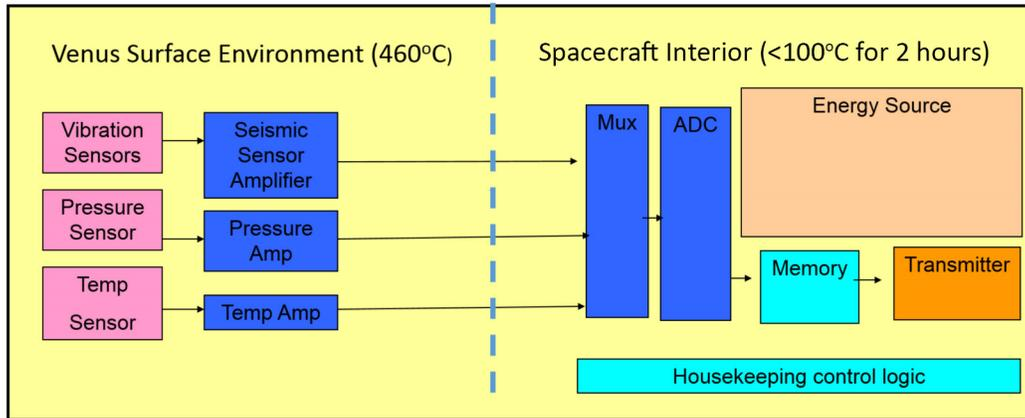
**Figure 5-7.** Block diagram of the Pathfinder experiment. The sensors and preamplifiers are exposed to the ambient Venus environment and the multiplexing; analog digital conversion and data storage is handled inside the lander.
