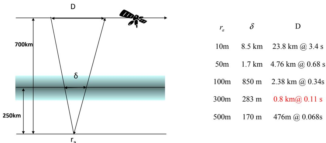
**Figure 7-7.** A resolution of a few km for the wave detection can be achieved with a meter-scale reflector.
