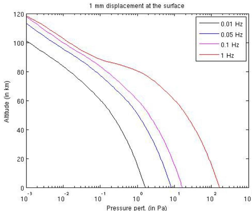
**Figure 6-4.** Amplification of a 1-mm ground motion as a function of the altitude, for various signal frequencies. This amplification is valid in the case of surface wave (planar wave), and underestimates the amplification near the source.
