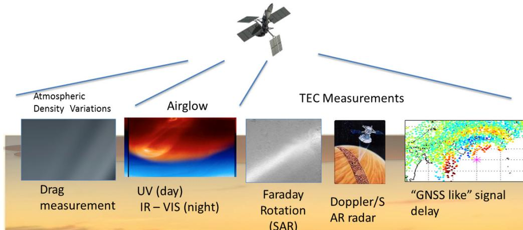
**Figure 7-1.** Orbital and ground-based observations that have been used for detecting terrestrial seismic events.
