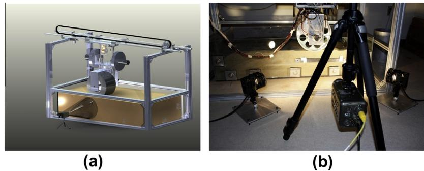
Fig. 1. CAD drawing of the terramechanics testbed showing the imager for PIV experiments (a). Actual PIV setup with the high speed camera and two flood lights (b).
