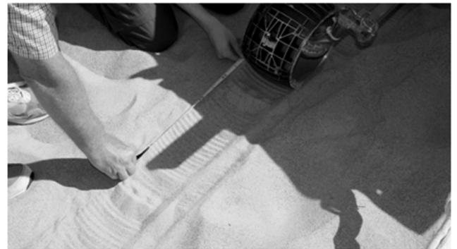
Figure 12. SSTB-Lite wheel slip measurement.
