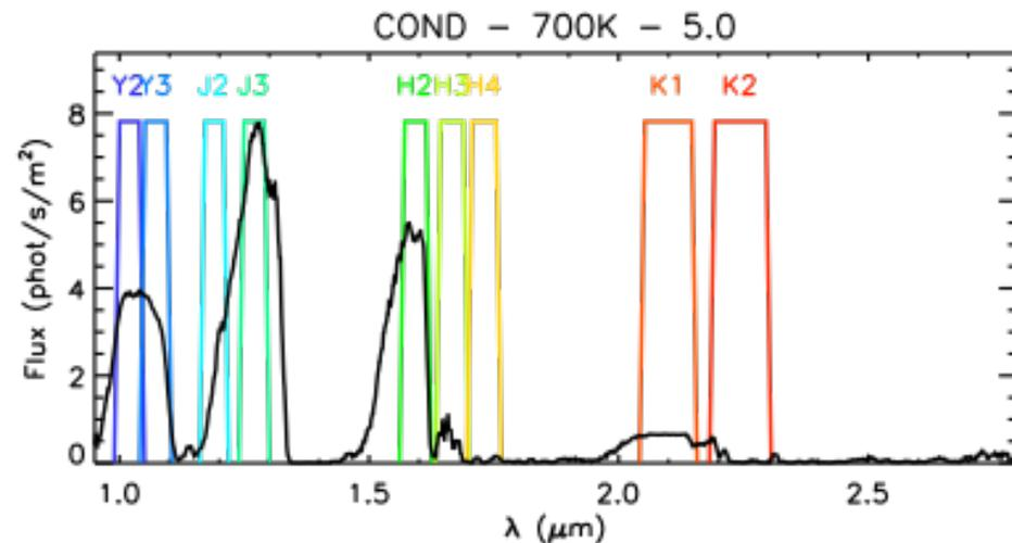
Example of SPHERE dual-band filters
