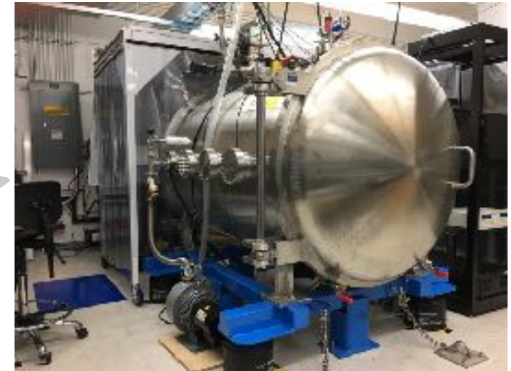
The Vacuum Surface Gauge interferometer provides a flight-like environment for DM characterizations
