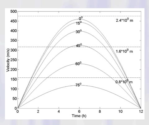
=> Minimal delta-V required to maintain shadow fixed on a telescope around that time.
