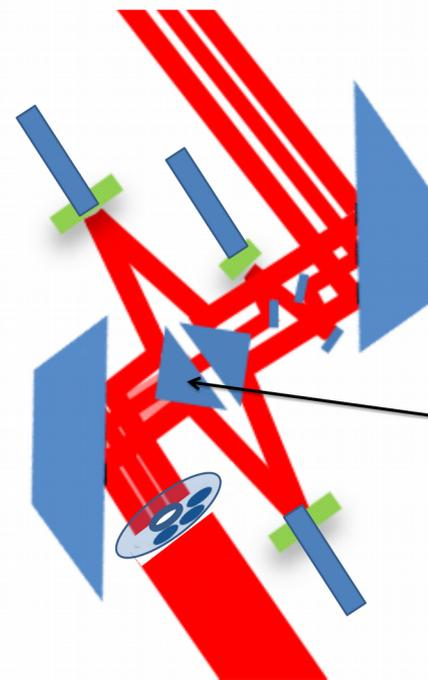
All pupils are exactly at the green planes and have the same path-length and pitch. After a second such relay the output pupil will be identical to the input pupil (SINE condition obeyed)
