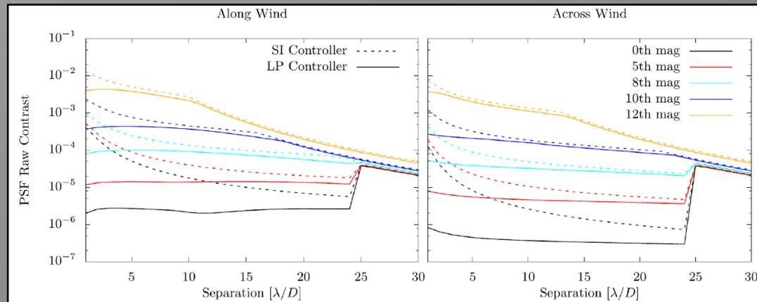
Contrast due to residual atmospheric speckles on a 6.5 m telescope.
