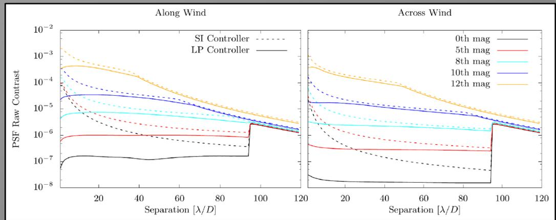
Contrast due to residual atmospheric speckles on a 25.4 m telescope.
