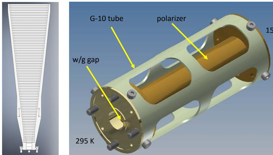
Figure 2: COMAP corrugated feedhorn (left) and circular polarizer (right)
