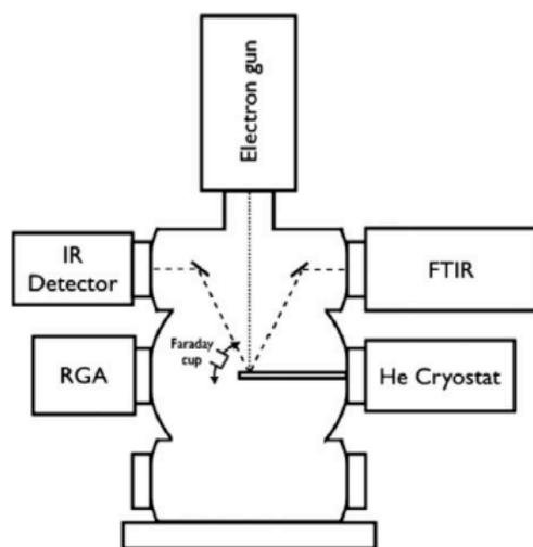
Figure 6. Diagram showing the chamber configuration.
