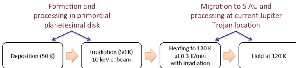
**Figure 7.** Typical experimental process for ice simulants.
