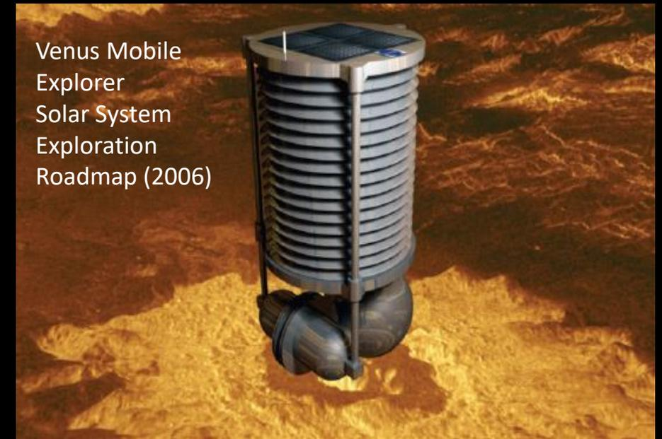
The bellows concepts was demonstrated but technical difficulties in long duration surface operation – power, refrigeration – had delayed further development of the VME concept
