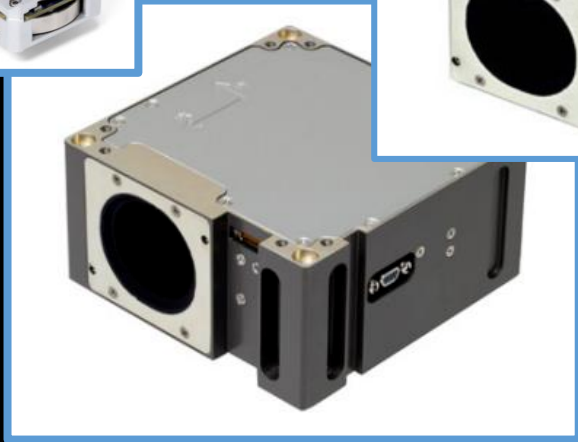
BCT XACT 0.015 Nms integrated ACDS Volume: 10 cm x 10 cm x 5 cm (0.5U) Used on ASTERIA and MarCO
