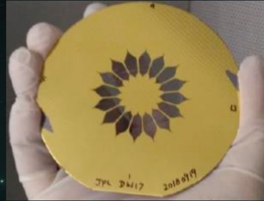
5-cm diameter Starshade etched in silicon
