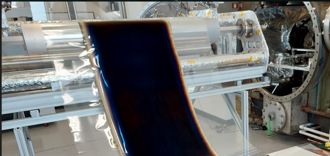
Photo of multilayer membrane 0.5 m wide coated by Zecoat under a Phase II SBIR. (Courtesy David Sheikh, Zecoat Corp.)
