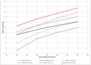
Figure 2: Velocity (AU/year) vs. A/m (m²/kg) for direct to perihelion (dashed) and Jupiter swingby (solid) trajectories for perihelions of 0.2 AU (black), 0.15 AU (gray) and 0.1 AU (red)
