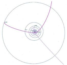
Figure 1: Two trajectory approaches to low perihelion to escape the solar system: Dotted – launch from Earth to perihelion, and then escape; solid – launch from Earth to Jupiter (not shown), then gravity assist to fly in to perihelion and then escape. In both cases sail is deployed after perihelion. Options for additional propulsion include high impulse chemical at perihelion and/or electric propulsion after perihelion added to solar sail.
