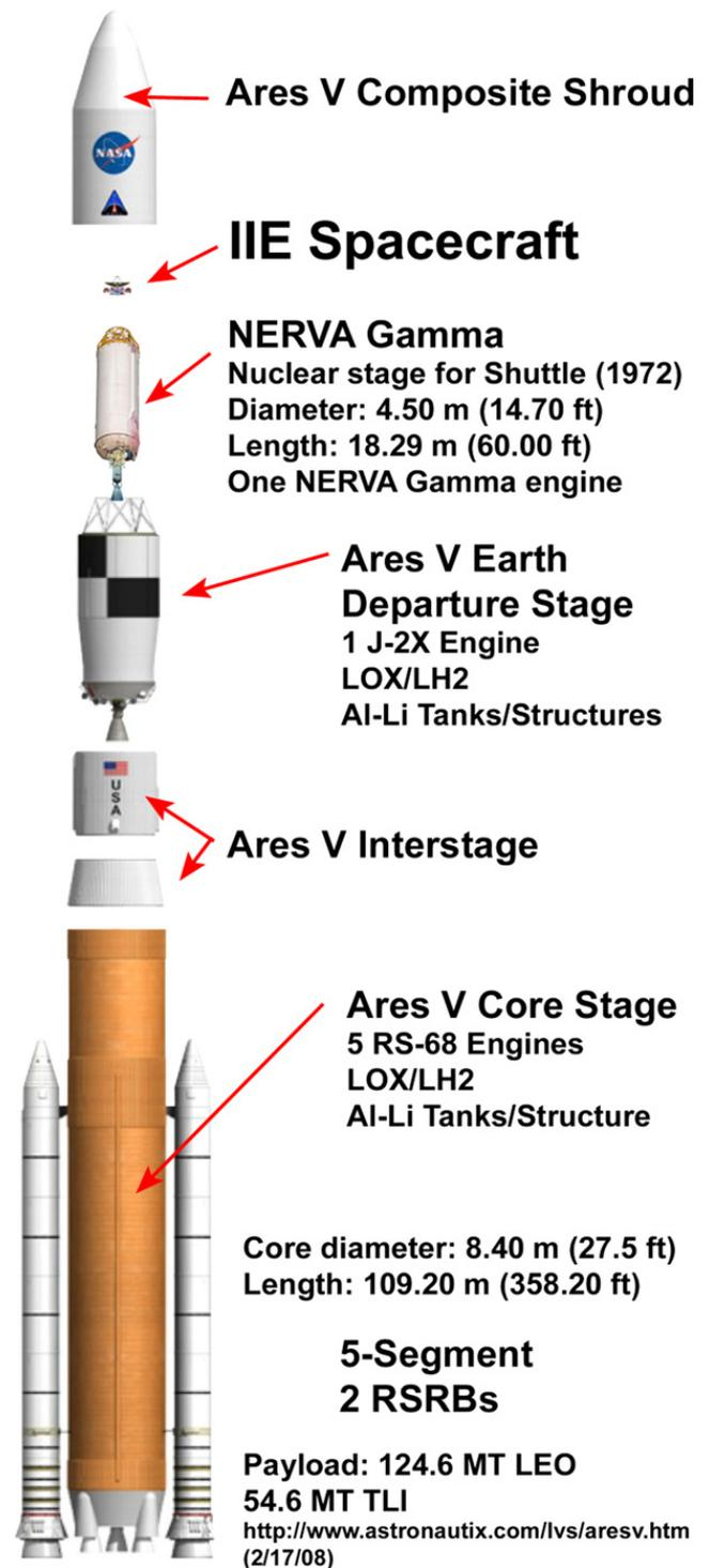
Fig. 4. Launch stack for an interstellar probe incorporating an NTR upper stage. Components, including the nuclear engine are approximately to scale. Drawings of Ares components © Mark Wade.
