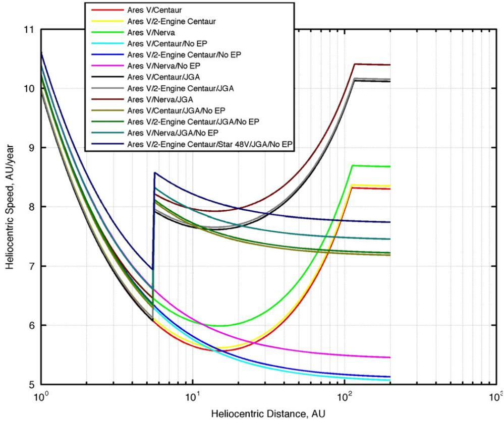
**Fig. 5.** Asymptotic heliocentric speed as a function of heliocentric distance for the thirteen different configurations considered. Note the slightly enhanced performance with the two-engine Centaur stage versus that for the stage with a single engine. The speed discontinuity at just greater than 5 AU is due to inclusion of a Jupiter gravity assist. “Burnout” of the REP stage can be identified by the slope discontinuities at just greater than 100 AU from the Sun.
