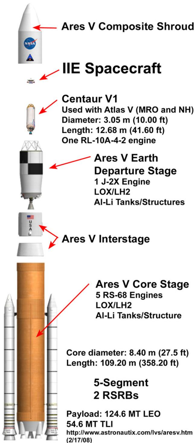
Fig. 3. Concept for Ares V with EDS and Centaur V1 used to propel an IIE spacecraft using REP. Drawings of Ares components © Mark Wade.
