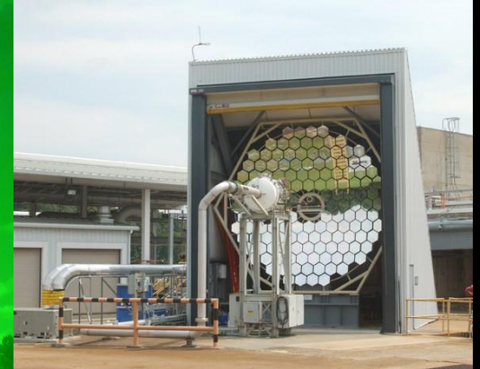
MSFC Solar Thermal Propulsion Test Facility ~10kW
