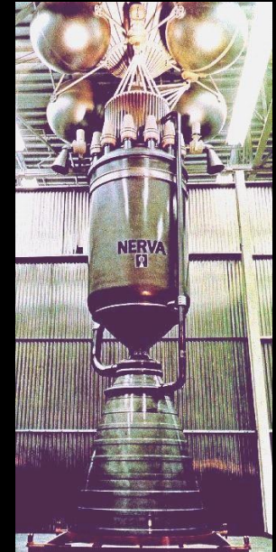
Nuclear Thermal Rocket Prototype from ~1970
