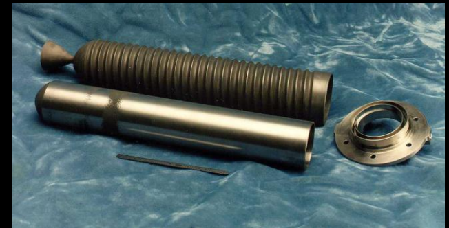
STP thruster made of 100% Tungsten
