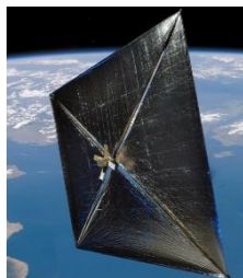
Figure 4. NanoSail-D solar sail. [3]
