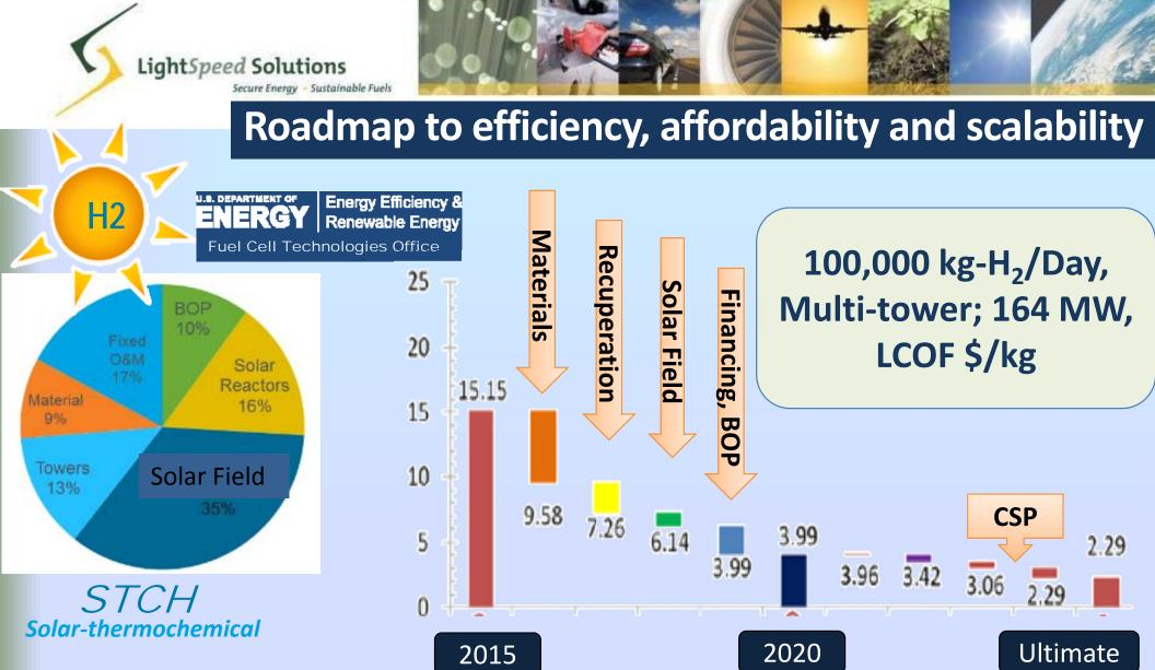
Solar-to-hydrogen conversion efficiencies > 20-30% likely needed to meet cost targets and that is true if photo-electrochemical or Solar Thermochemical.
