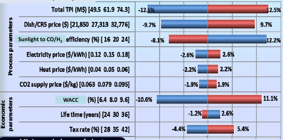
Minimum balance of plant optimization, baseline analysis: **Better separations Heat integration** One step syngas to fuel synthesis
