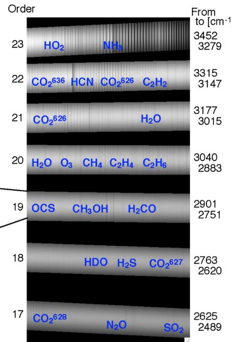
A2. Spatially resolved spectra of all critical atmospheric gases are obtained simultaneously for each pixel along the slit (12 km pixels at nadir). Each pixel along the slit maps into a spectrum on the 2Kx4K detector. In one Mars' day, 50% of the planet can be mapped.
