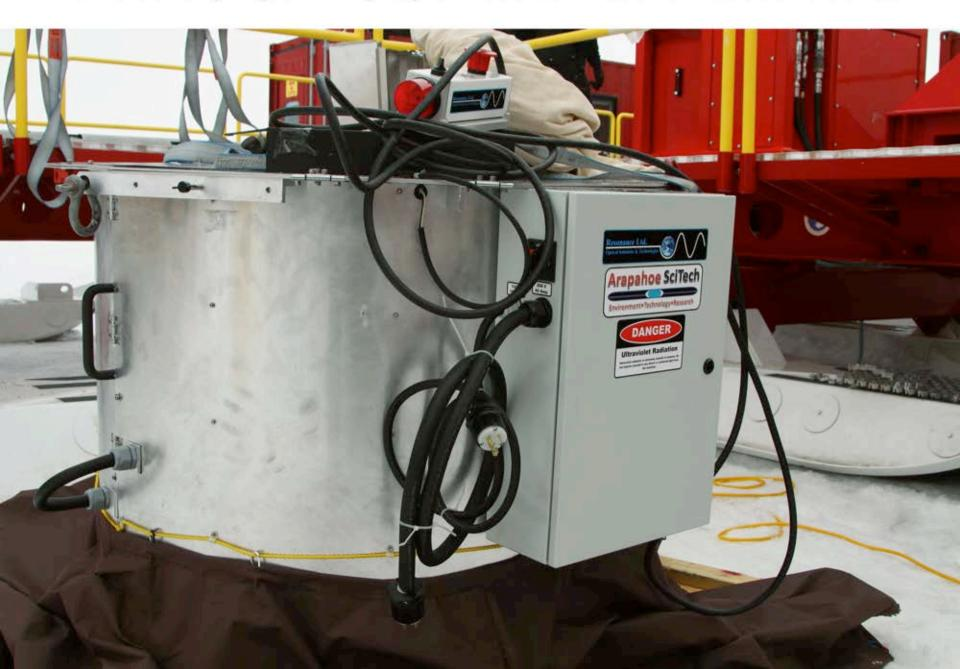
Looking Down into the WISSARD Borehole through the UV-C Collar used for Decontamination of Hoses and Cables [12 Germicidal UV-C Mercury Amalgam Lights]
