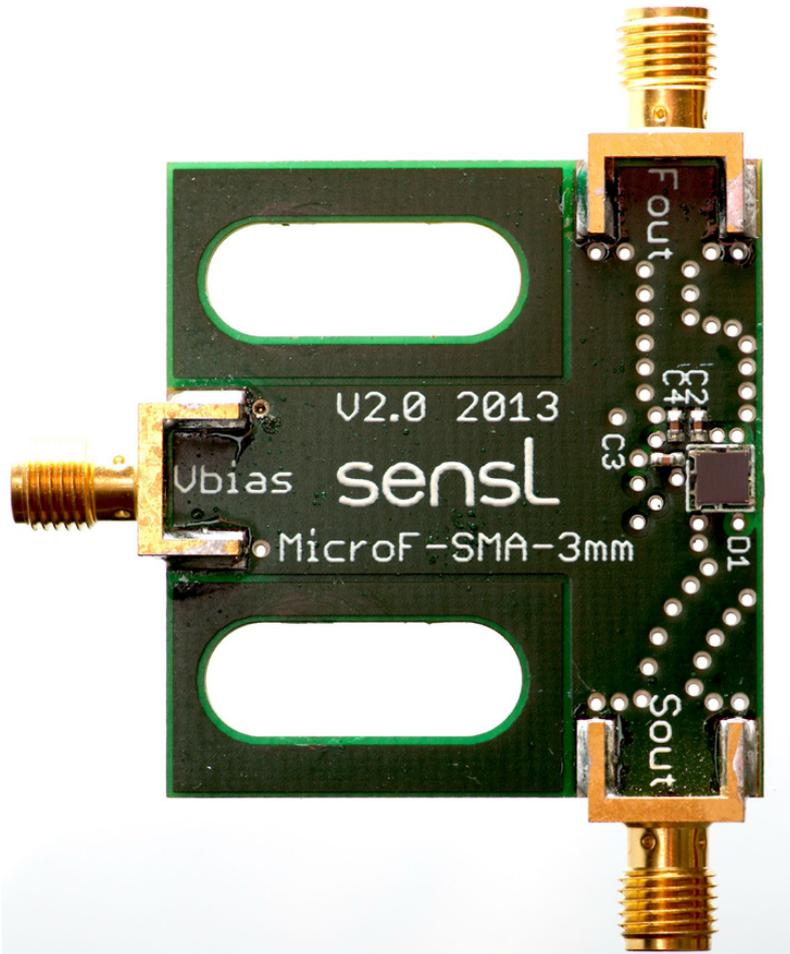
Detector: Sensl MicroFM-SMA-10020
