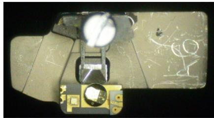
Alignment of laser to resonator
