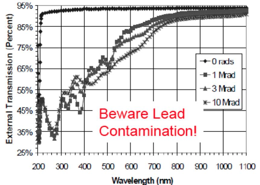
Figure 24. Transmission measurements of a Schott 193 nm eximer grade synthetic monocrystalline CaF<sub>2</sub> window after exposure to gamma radiation ( $t = 9.94$  mm).
