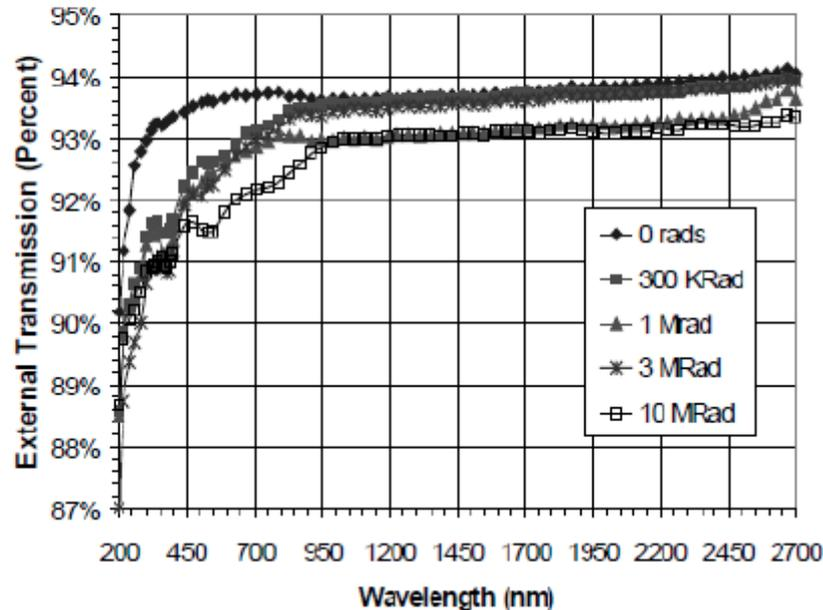
Figure 23. Transmission measurements of a Schott 157 nm eximer grade synthetic monocrystalline CaF<sub>2</sub> window after exposure to gamma radiation ( $t = 7.065$  mm).
