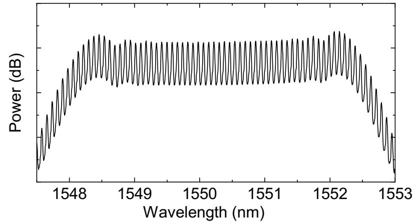
Features: Wide mode spacing, tunable, mWs per mode, COTS + scalable fabrication, retrace
