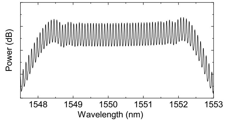
CW laser is the center of comb
