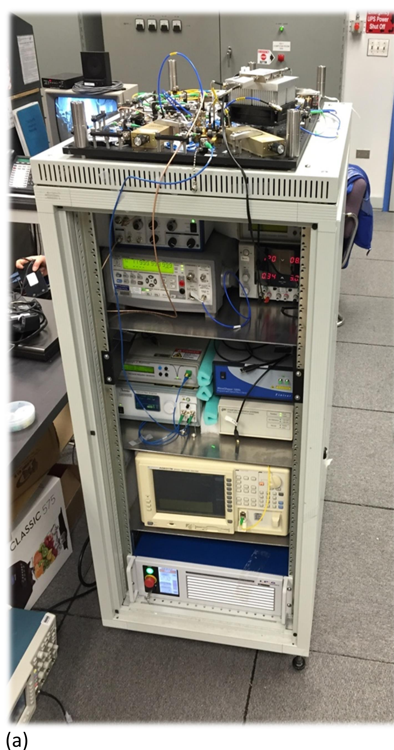
Fig. 2. (a) LR-EOFC breadboard (top of rack) and supporting equipment. (b) Comb line intensity stability: variation within 2dB over five days and power on-off cycles. (c) Allan Deviation measurement of reference laser. Stability better than 30 cm/s is achieved.
