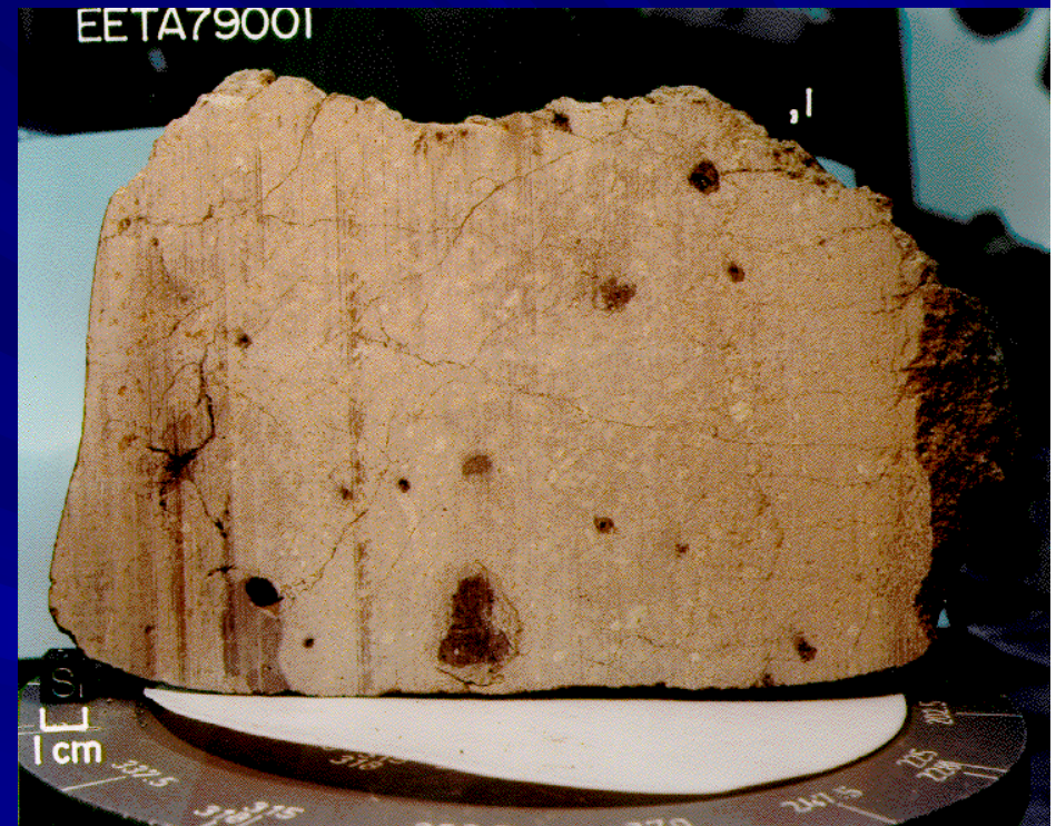
Martian meteorite Elephant Moraine 79001, with its shock-produced glasses (dark patches) full of Martian atmospheric gases.
