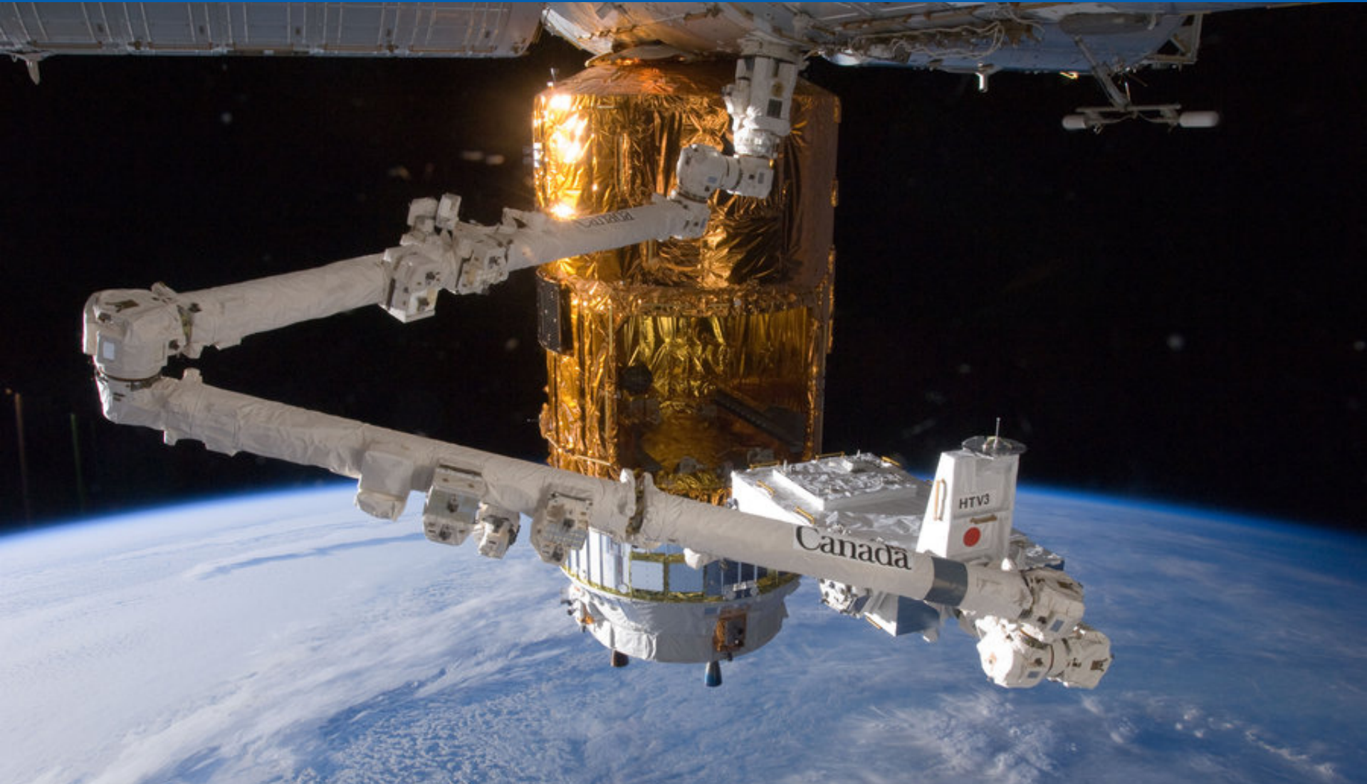
Space Station Remote Manipulator System (Canadarm2)
