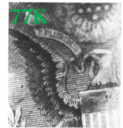
Figure 7.6 Image taken while CCD was submerged in liquid nitrogen.
