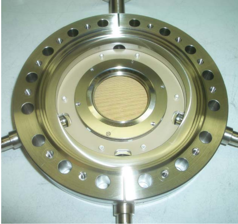
50 mm Cross Strip anode open face detector, MCPs not installed.
