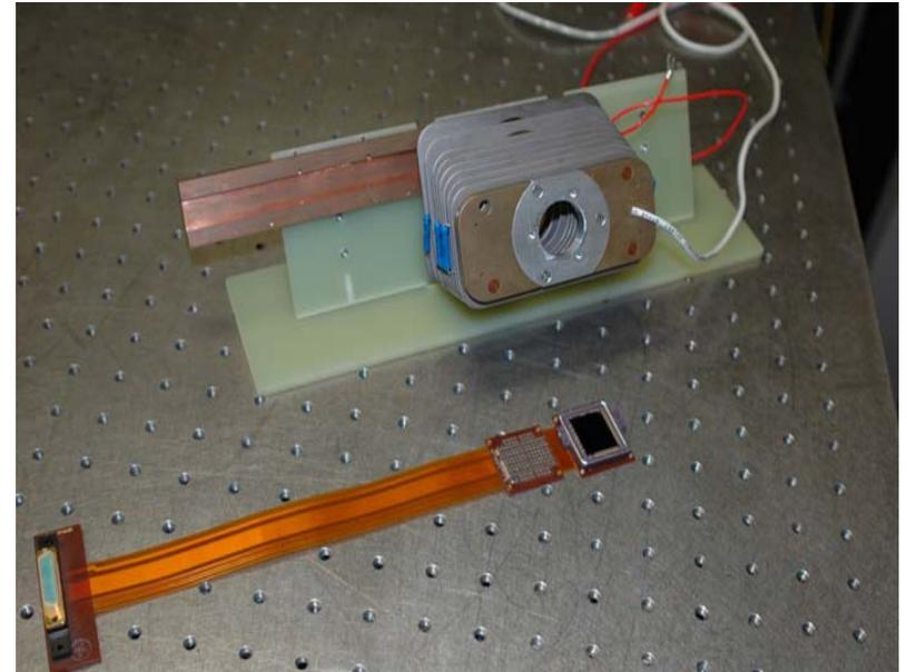
Bread-board electrodes with ISIE11 EBCMOS Sensor and Flex cable harness.
