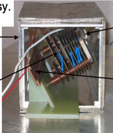
Photocathode sits on a "top-hat" piece, to be bolted back here.
