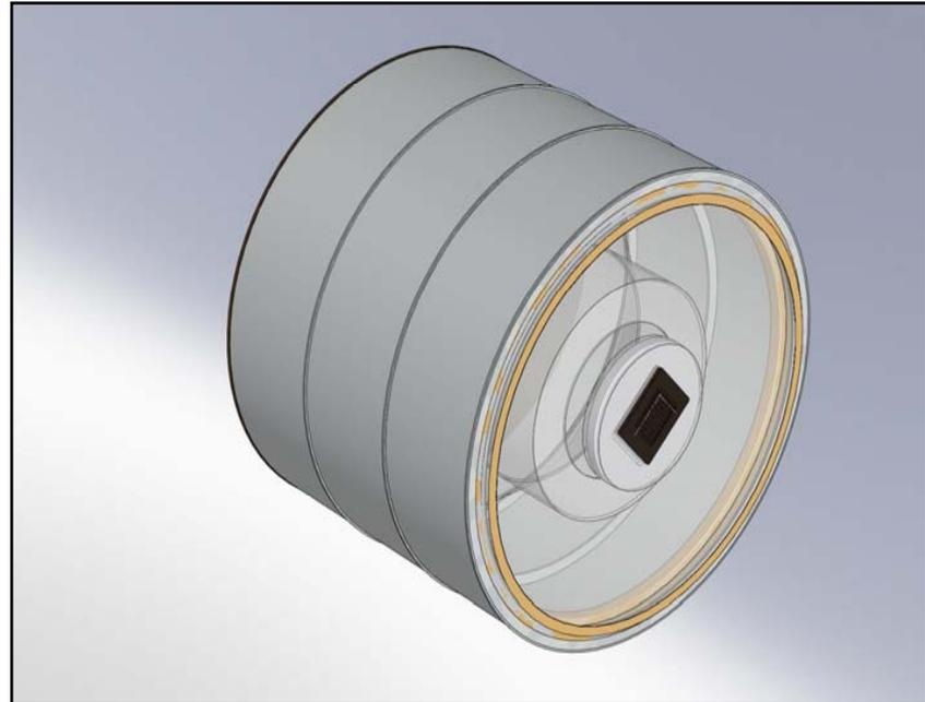
Bottom-left – CAD representation of high QE, high Etendue tube design, Kovar-Ceramic, MgF<sub>2</sub> window, In-Bi seal.
