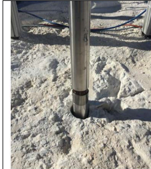
PLANETARY DEEP DRILL BORES THROUGH GYPSUM ROCK DURING ITS FIRST FIELD TESTS
